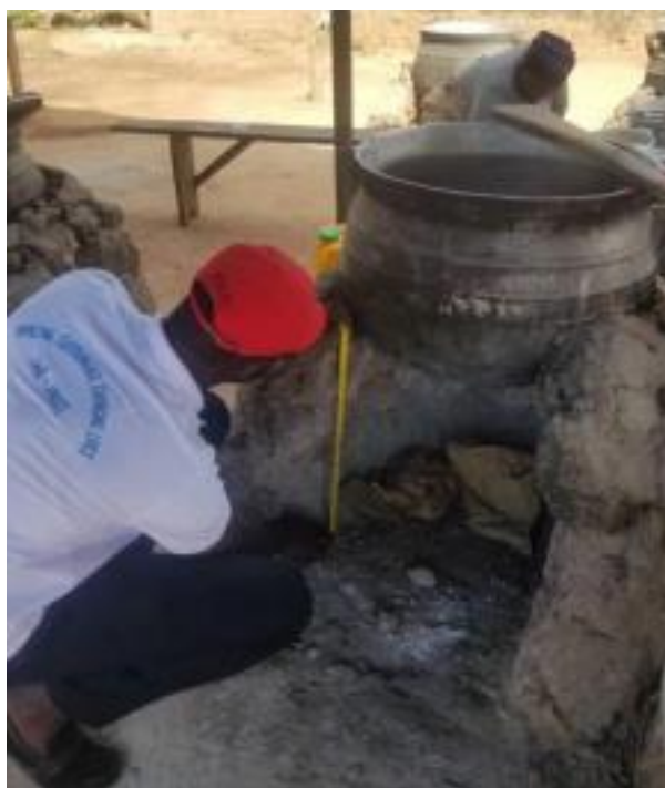
Measurement of a fuel opening of a typical traditional cookstove in Ullo S.H.S.
