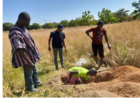
Figure 3: An image showing trial pits being dug
