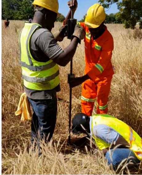
Figure 6: An image showing DCPT test in progress
