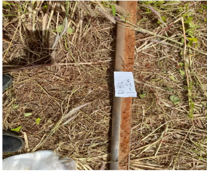
Figure 5: An image of a sample obtained by Auger drilling
