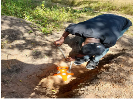
Figure 2: An image showing the trial pit being logged
